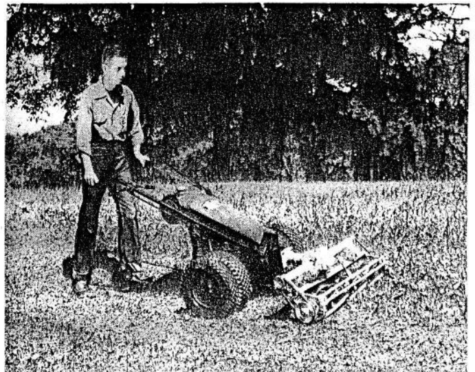
Dual wheels, quickly and easily attached, make mowing of steep slopes, terraces, fast and easy.
